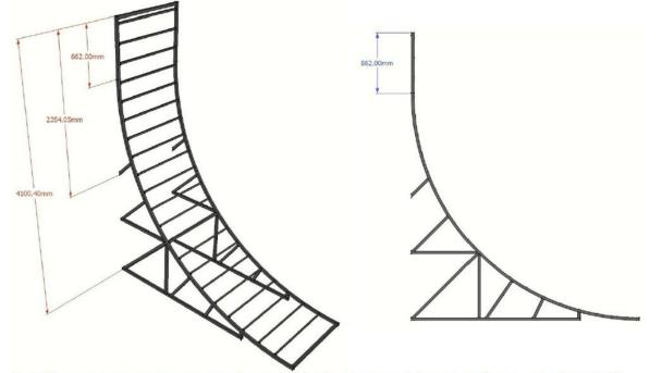
Use the Measurements from the Normal Extension. You will notice that the only difference between them is the vert section which is 862.00 mm and not 561.2 mm
