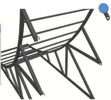
Materials for the extension are basically the same as the normal transition. The only difference here is that the Square tube for the bends is longer.
