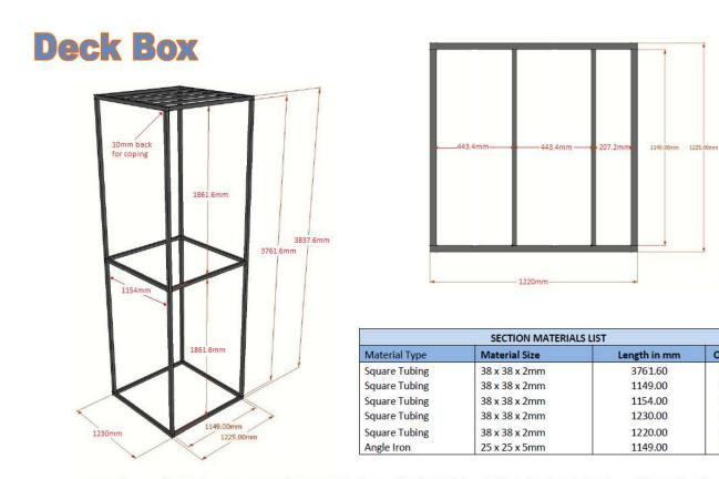
Note: The one side of the box is 1,220 mm. The reason behind it is so the ply wood sheet will fit and so the metal surface will hang off on the one side by 5mm to cover the gap between the frame and the coping. Look at the coping detail for more information on this.
