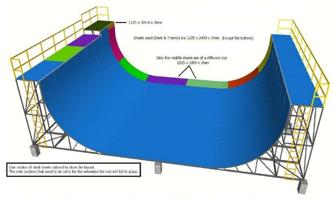
Note: All sheets used are the same size except for the two sheets used in the flat bottom. The Ramp was designed around these sizes so that it wouldn't be necessary to cut the steel sheets. Cutting sheet metal is a serious pain.
