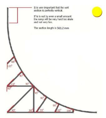
Only the longest edge length is given for the frame supports to allow for the angles to be cut. These angles is only given here as a reference. Too my knowledge they should be correct but make sure by doing some measurements of your own first after building the main structure.
