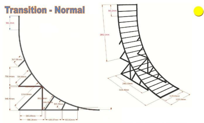
Note: The transition has a radius of 10.5 ft / 3,200.4 mm and the length of the square tube measured on the inside of the bend is 5,027.18 mm. The blue measurement indicates the amount of vert (1.5 ft / 561.2 mm)
