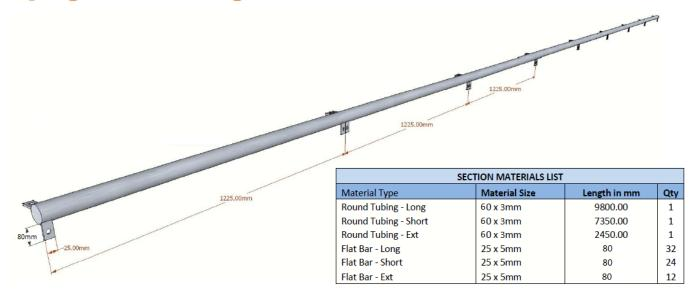
The steel used to fix the coping (60mmx3mm pipe) to the ramp is 25x5 mm flat bar.
